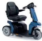
An intuitive ergonomic wig-wag control sets the new standard of scooter drive controls. Information of your journey - distance and speed is easily displayed on the backlit LCD control unit. The Elite<sup>2</sup> XS is designed for comfort with the unique adjustable rear suspension, adjustable seat, gas strut adjustable tiller and delta handle bar.
