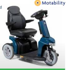
Full front and rear suspension and 14" wheels gives a comfortable ride in everyday terrain. A clear and easy to use LCD display gives control over driving profiles, LED lights and turn signals and stores information on distance travelled. Ride in comfort with an easily adjusted central steering drive control, a height adjustable 360° swivel seat with slider and adjustable armrests.
